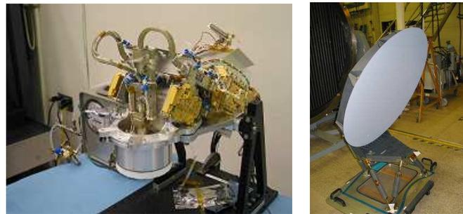
Figure 4 : OSTM/Jason-2 AMR Instrument and Antenna
