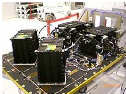
**Figure 3** : OSTM/Jason-2 Posidon-3 Instrument
