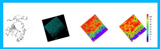
*Figure 14.* (from left to right) location of the scene shown; true color image of Landsat; Landsat sea ice concentration; and S-NPP VIIRS ice concentration at 12:09 UTC on May 27, 2013.
