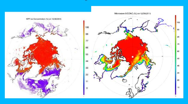
*Figure 13*. Ice concentration for daily ice concentration composite from VIIRS (left) and from microwave using NASA team algorithm (right) over the Arctic on December 9, 2015.
