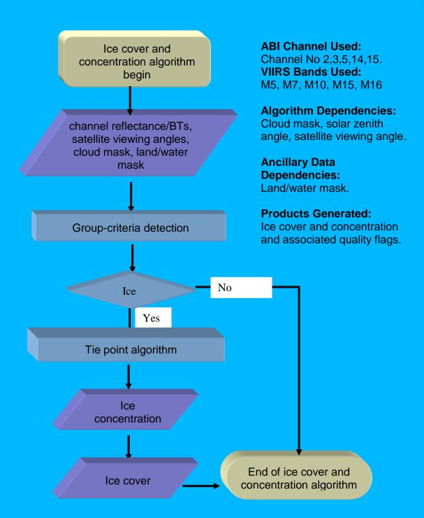
Figure 1. High Level Flowchart of the ice cover and concentration algorithm illustrates the Main Processing Sections.
