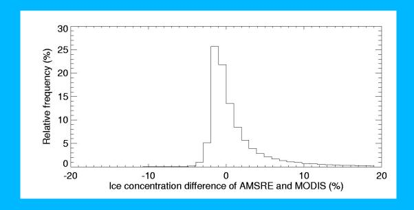
Figure 8. Frequency distribution of ice concentration difference between AMSRE product and retrievals using this algorithm based on selected 41 clear day MODIS data in four seasons in 2007 over the Arctic Ocean.
