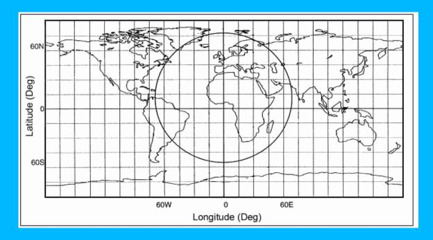
Figure 5. MSG Telecommunications coverage area.
