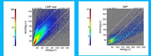
Figure 26 Comparison of Water Path for Days 230-239 in 2006 derived from MODIS (MYD06 and MOD06) products and from DCOMP algorithm. Left image shows results for water phase (LWP), right image for ice phase (IWP). Accuracy and precision of the comparison are shown in the figures. Specs ranges are added as white lines in the figures.
