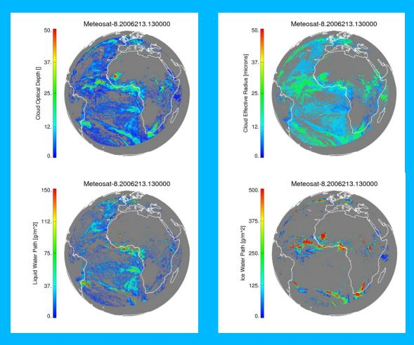
Figure 14 Results of the retrieval for 1 August 2006 13:00UTC for SEVIRI. Upper panel shows optical depth (left) and effective radius (right). Lower panel shows liquid water path (left) and ice water path (right).
