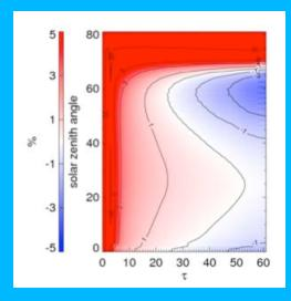
Figure 10 Potential error in percent if Rayleigh correction is not applied as a function of  $\tau_c$  and solar zenith angle. Observation angle is 43 degrees and effective radius is 8  $\mu m$ .
