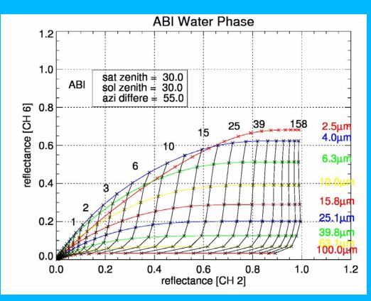
Figure 7 Theoretically computed cloud reflectance function for water phase of GOES-ABI channels 2 and 6 (DCOMP channel 1 and 3) for an arbitrary geometrical observation constellation.
