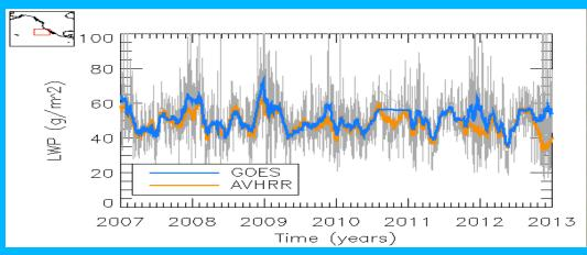
Figure 19 Time series of Liquid water path from DCOMP results in PATMOS-x data set in comparison to GOES-West results.
