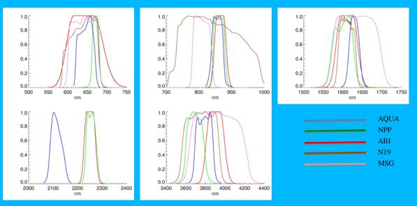
Figure 1 Channel response functions for DCOMP channels 1-5 for five sensors.
