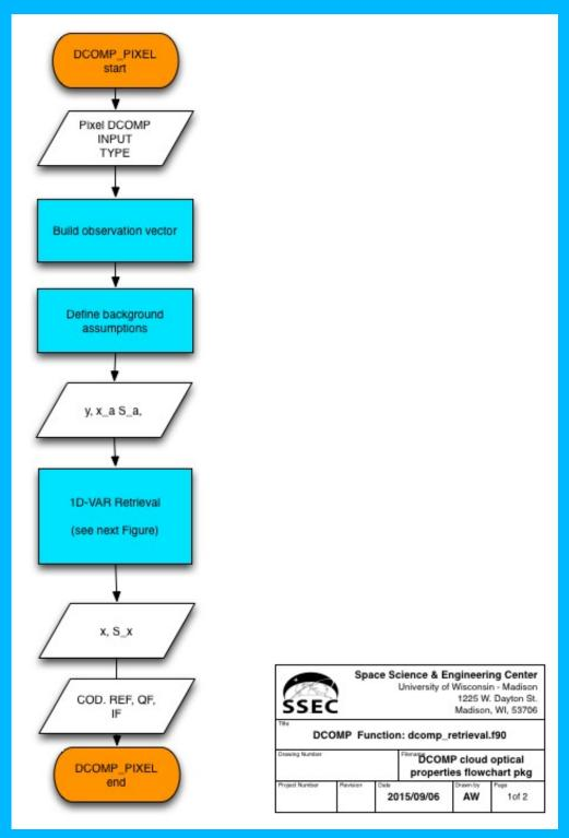
Figure 3 DCOMP: Pixel-based flow chart
