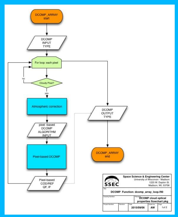
Figure 2 High-level flowchart of the DCOMP algorithm.
