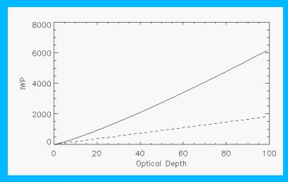
Figure 5 Comparison of Heymsfield method to a traditional method (dashed line) of calculating the ice water path from optical depth.
