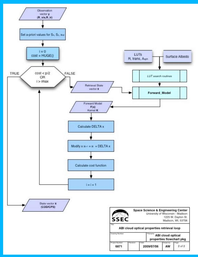
Figure 4 Flow chart of 1D-Var inversion retrieval loop.
