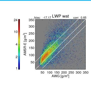
Figure 27 Comparison of AWG-DCOMP Liquid water product to AMSR-E for a two-day period (24-25August 2006) as a 2D histogram.
