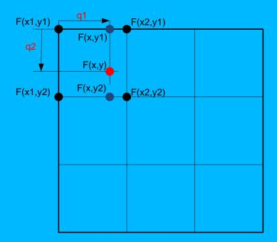
Figure 9 Pictorial depiction of LUT linear interpolation in both one and two dimensions.
