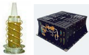
Figure 5 : Jason-3 DORIS Receiver Antenna and Instrument
