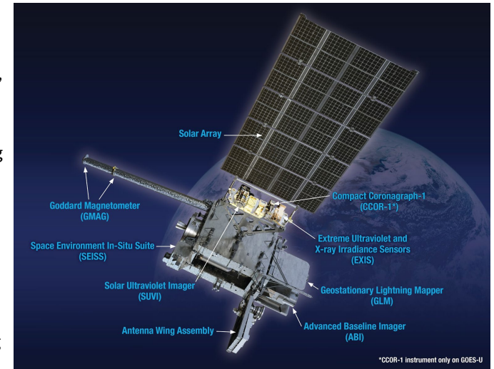
Figure 2. GOES-R Series satellites are composed of 6 (7 on GOES-19) instruments, and powered by a solar panel array.
